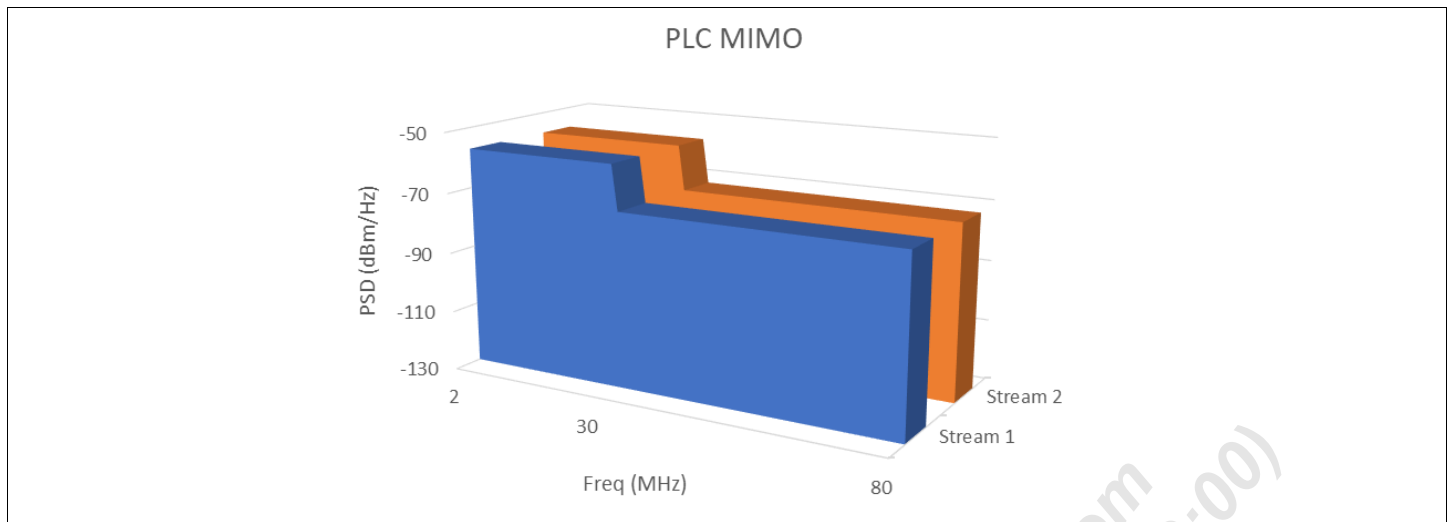
Figure 1: PSD Levels Description for MIMO PLC Supported in Spirit HN
