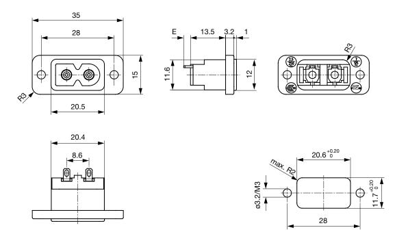
E: Solder terminals long: 7.3 mm (L=8.5 mm)
